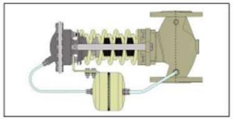
To adjust inlet pressure, use adjustment nut (illustrated in assembling plan). If you turn it clockwise inlet pressure increase and vice versa. Before starting up, put the fluid through the pressure to remove any dust and impurities that are present in the line, as well as areas where sealing is not appropriate. Note that this pressure should not exceed 1.5 times the normal pressure of the body because it damages some of the valve parts, including the actuator.
